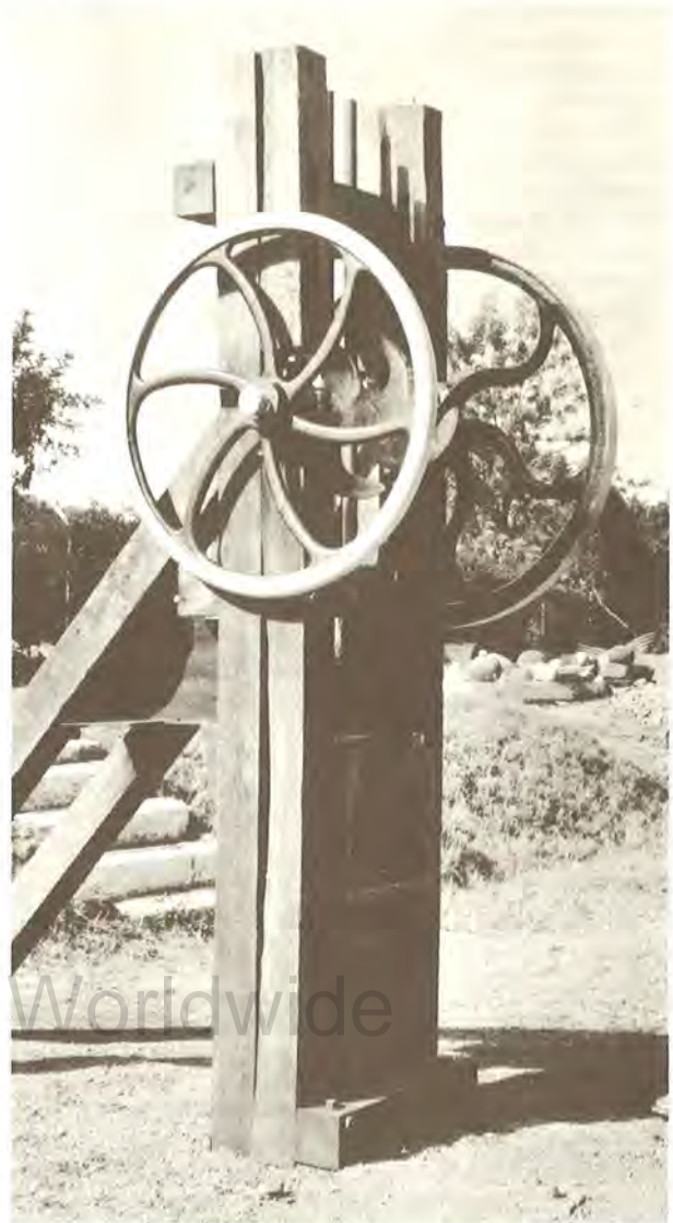
3-stamp hand-operated battery brought into Rhodesia before the turn of the century from Mozambique by Count Rezende to crush gold-ore near Penhalonga
