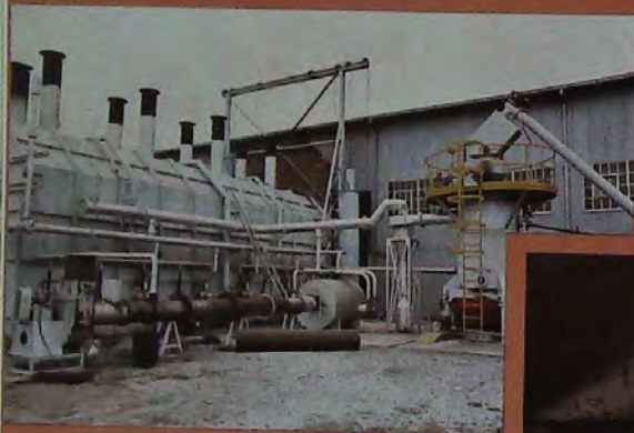
Another important by-product of coal is producer gas, which is given off when coke is burnt. Plants for the production of this clean fuel are being built in Rhodesia and are already in use in industry (above). In such units the coke provides initial heat as it burns, and the gas collected is also used for heating purposes (right). This extended use of coal, with various processes reaping many forms of fuel as by-products, underlines its importance as a portable and versatile form of energy.
