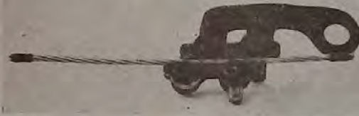
Aluminium conductor gripped by "come-along" clamp.
