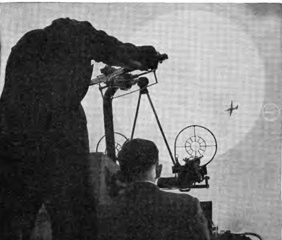
Image of a four-engined aircraft traverses wall of the Portobel, while the gun crew (foreground) attempt to register hits. Results are visible to their instructor. On the extreme left is Commander Stevenson, of the Indian Navy, who had come to watch a demonstration.
