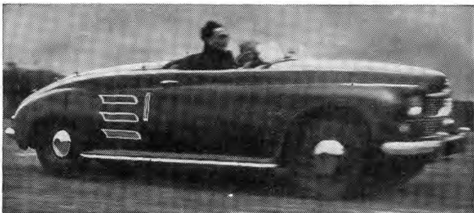
At nearly 90 m.p.h. on a rough concrete track it was difficult to separate tyre and exhaust noise. At idling speeds the engine sounded like any other gas turbine warming up and at no time was turbine noise particularly apparent. During fierce acceleration tests the sound rose to the familiar, high-pitched scream of a jet aircraft.
