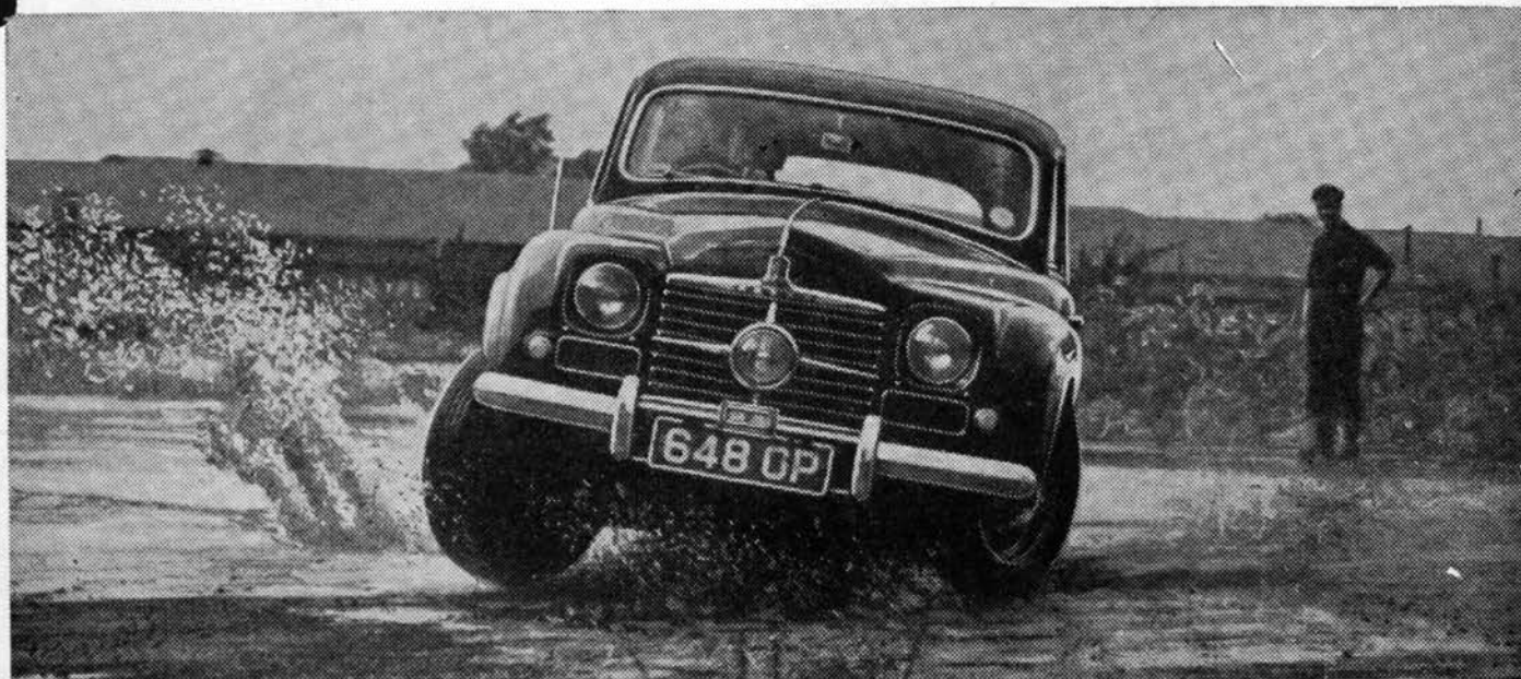
Dirt flies as a test car is driven on to the skid track. It is a tarred road well sprayed with water.
