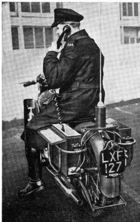
Latest addition to Scotland Yard is a fleet of motor-cycles fitted with two-way radio equipment, for use by the Metropolitan Police Patrols. Approximately 35 machines will be in use to control Festival of Britain traffic and later there will be a squad of 200. Each is fitted with a five-foot aerial and when a call is put through from Scotland Yard an orange light flickers on the dial attached to the handlebars and a buzzer sounds. The policeman can then communicate direct with Scotland Yard by means of the telephone as shown above.
